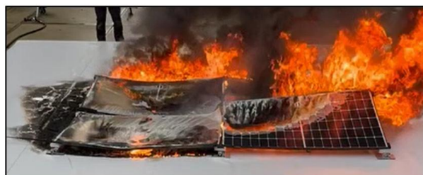
Figure 2 – Baseline test with PVC membrane, two layers of glass fleece and EPS insulation. 10 minutes after ignition. Test 1 in the phase 1 report [12].
